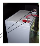
Connect the two ring terminals on the connector end of the cable to the battery. The battery charger or solar panel should be installed at this time.
