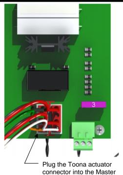
connector on the circuit
