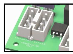
Applies battery voltage directly to motor to open gate (will not close gate) if control board fails. User must unplug before gate opens to maximum travel or the 15 amp fuse will open. Fuse should be checked before returning gate to service.
