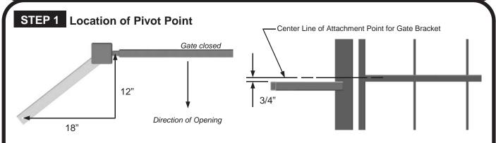
Weld the pivot arm to the hinge post or other solid surface using the dimensions shown. Pivot arm must be level for proper operation.
