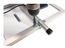
Step 2: Screw u-brackets onto panel with the included self-tapping short screws. Be sure to use a 5/16" hex bit in your screwdriver.
